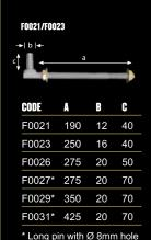
for securing gate to hinge.
